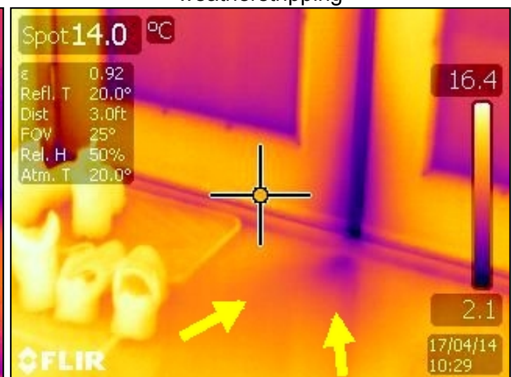
Heat loss at exit doors due to poor weatherstripping
