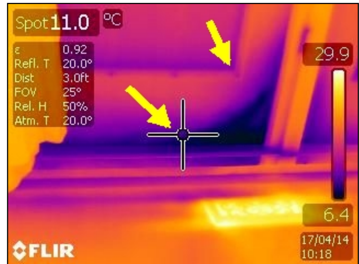
Heat loss at exit doors due to poor weatherstripping
